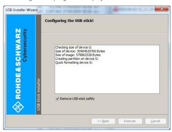
When the message "Configuration successfully completed" is displayed, a bootable USB mass storage device for installing the new LCOS FX system image is created.
